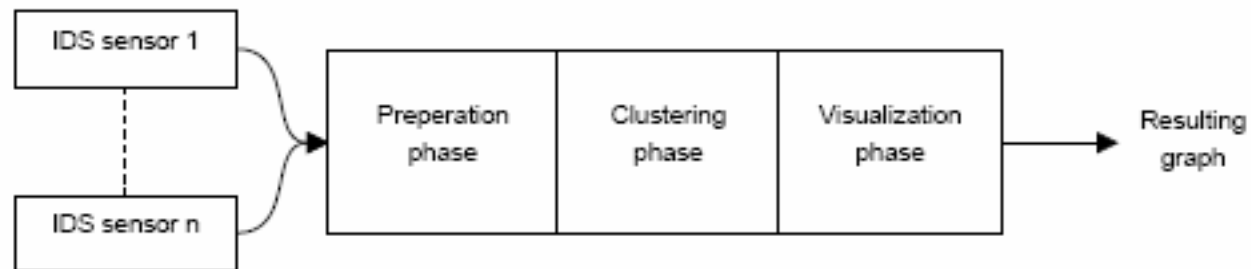
Figure 1: Diagram of the three phases of the system
